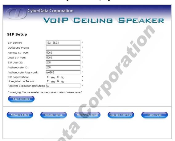
2. On the SIP Setup page, enter values for the parameters indicated in Table 2-7.
